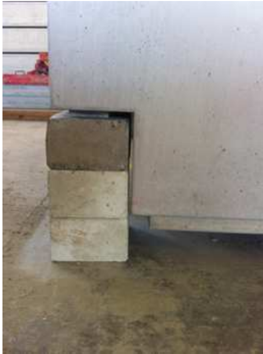
Photograph 5: Support at the panel end during the full scale test
