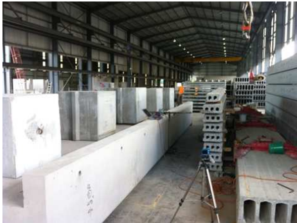
Photograph 6: Full scale load test at precast factory
